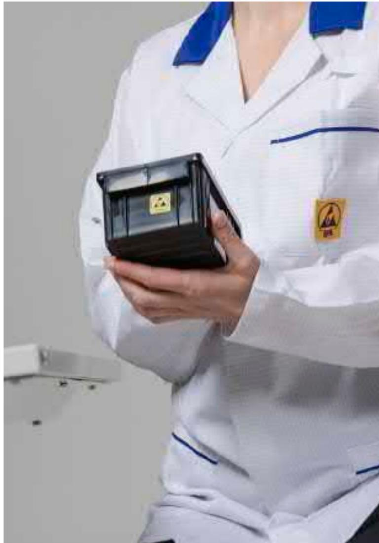
Though the bags are safe havens for sensitive components, you should not totally depend on them as one of them might contain a small hole or might not have been sealed correctly, which could result in damaged components. It is therefore important that the trolleys and bins being used to transport sensitive components and parts around the factory are ESD protected, as they ensure ESD protection, enhance safety and reduce the risk of potential damage.
