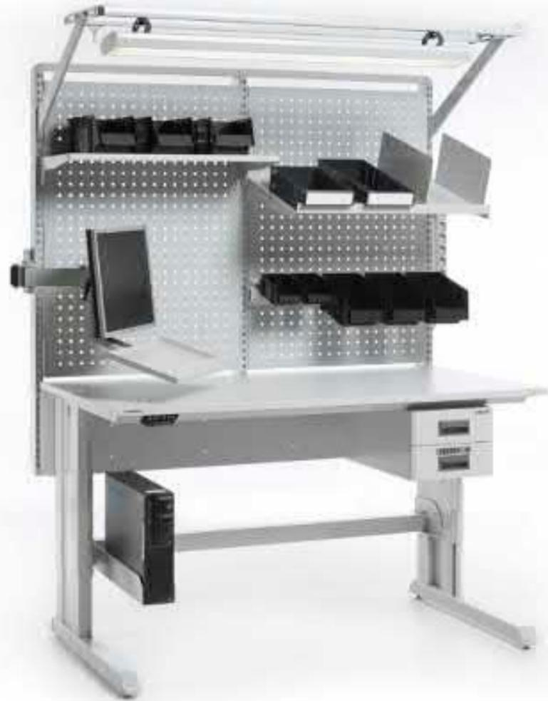
There are two types of ESD-protected workbenches. When a workbench is semi-conductive through its structure, ESD protection is in place as soon as the bench's feet touch an ESD floor. This is very simple and easy. Other benches always require wiring to a common point ground.
