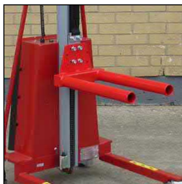
Double Spindle – EP06 Ø50 x 500mm (260mm centres)
