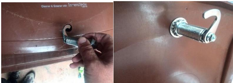
3 Remove nut and washer, insert lock and arm through hole. Replace washers and nut, tighten with shifting spanner or similar.
