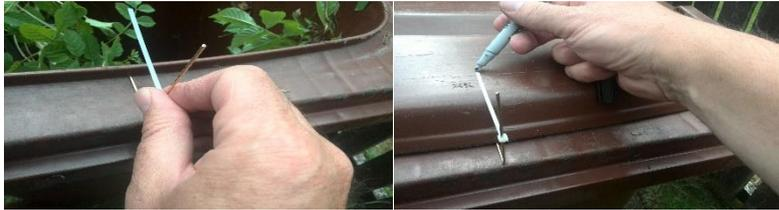
2 Gentle close lid in top of indicator arm. Lower plastic arm down on to the bin lid. Keep it level and mark at the end of plastic strip with a felt tip pen. Drill on mark with 22mm hole with hole cutter.
