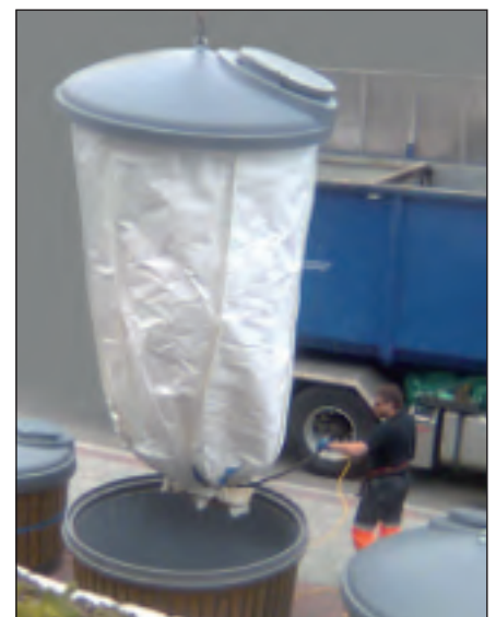
Fast emptying with the "One Hook System"
